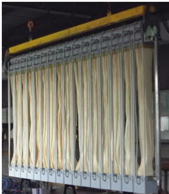
Figure 2: Typical MemRACK™ nylon Rack Assembly fitted with 16 (sixteen) MBR Membrane Filtration Modules and suspended from a Rack Lifting Beam (yellow).
