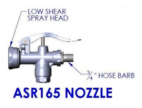
Recommend pressure for max flow 20-25psi GPM 6.6 at 14.5psi GPM 9.0 at 22psi
